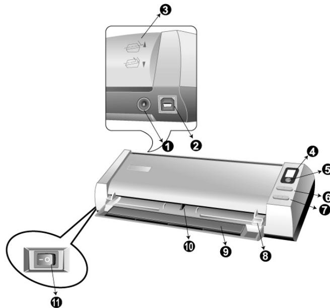
1. **Power Receptor:** It connects the scanner to a standard AC power outlet by the included power adapter.
